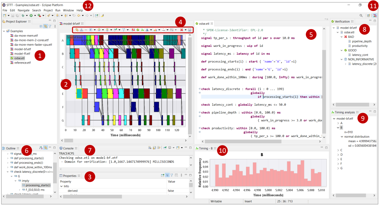
Fig. 3: Overview of the Trace user interface. The file explorer view (1) shows the trace files (Gantt-chart icon) and in this case a single specification file (see Sec. 4) with the green checkmark icon. The Gantt-chart viewer (2) shows trace files. Parts of a trace file – events, dependencies, claims, and signal fragments – can be selected and their properties including the attributes are then shown in the properties view (3). Each Gantt-chart viewer has a toolbar (4) with items to apply techniques, such as the filtering, coloring and grouping visualization techniques. The various editors support syntax highlighting etcetera. In (5), a property specification file is shown. The outline (6) shows the structure of the property in the highlighted line. A specification can be checked on a trace file (invoked from the toolbar (4)). Logging of the verification algorithm is written to the console view (7), and the results are shown in the verification view (8). Another type of analysis is the timing analysis, for which the results are shown in a timing-analysis view (9) and a timing-histogram view (10). There is also an Eclipse perspective (11) that gives a default layout for all relevant views. The layout shown is not the default; various views have been relocated (by drag-and-drop) to convey as much information as possible in a single screenshot. Finally, the help menu (12) gives access to documentation of the Trace tool.
